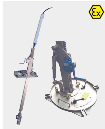
Lance system Manually extendable, tilting lances. The nozzle standoff distance is adjusted by a crank drive and chain.
