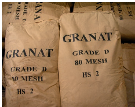
Abrasive material: garnet sand and garnet in a grain size of 0.1 – 0.2 mm
