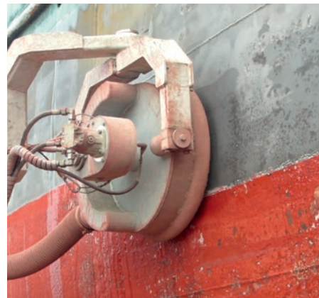
The Dockboy is a semi automatic vehicle primarily for working on ship hull bottoms or similar surfaces.
