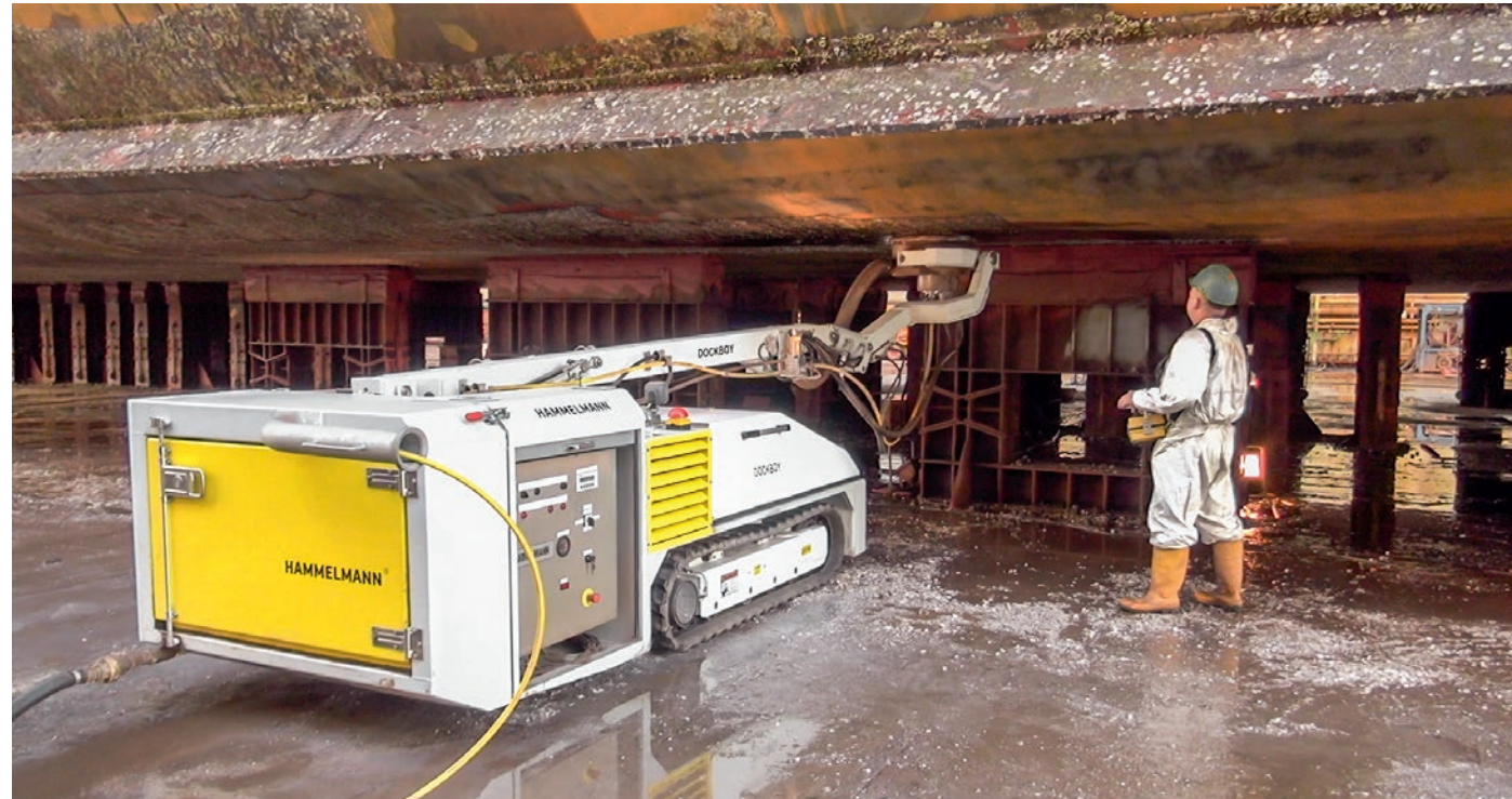
The Dockboy is a semi automatic vehicle primarily for working on ship hull bottoms or similar surfaces.
