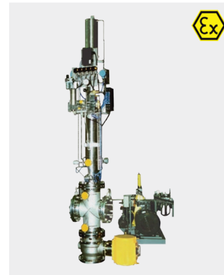
Gastight lance system Four-stage telescopic lance driven by high pressure water. The cleaning device is controlled and monitored by a freely programmable PLC.
