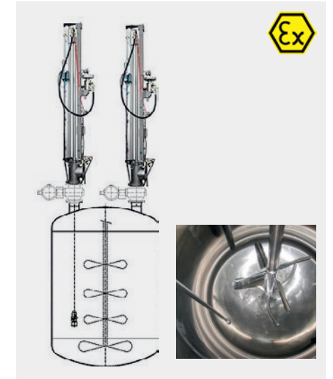
Twin lance system The entire cleaning device is powered by high pressure water and oil-free compressed air. (With chain drive as an alternative for a stroke of 4.5 m or more.)
