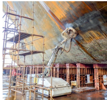
The Dockboy is a semi automatic vehicle primarily for working on ship hull bottoms or similar surfaces.
