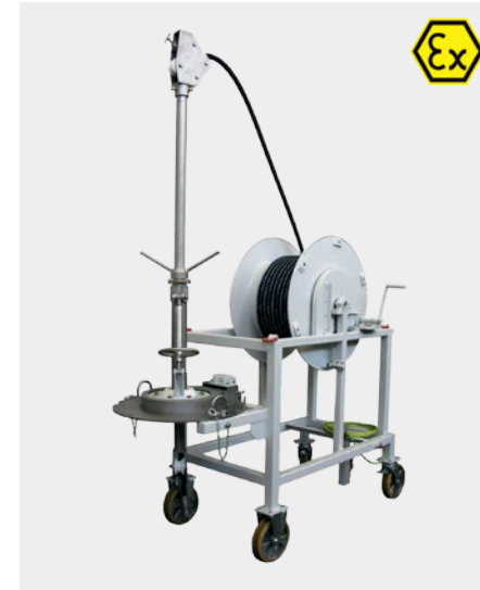
Lance hose system The lance can be rotated, swivelled and extended and is attached onto a manhole. The tank cleaning device is lifted and lowered using a crank handle.
