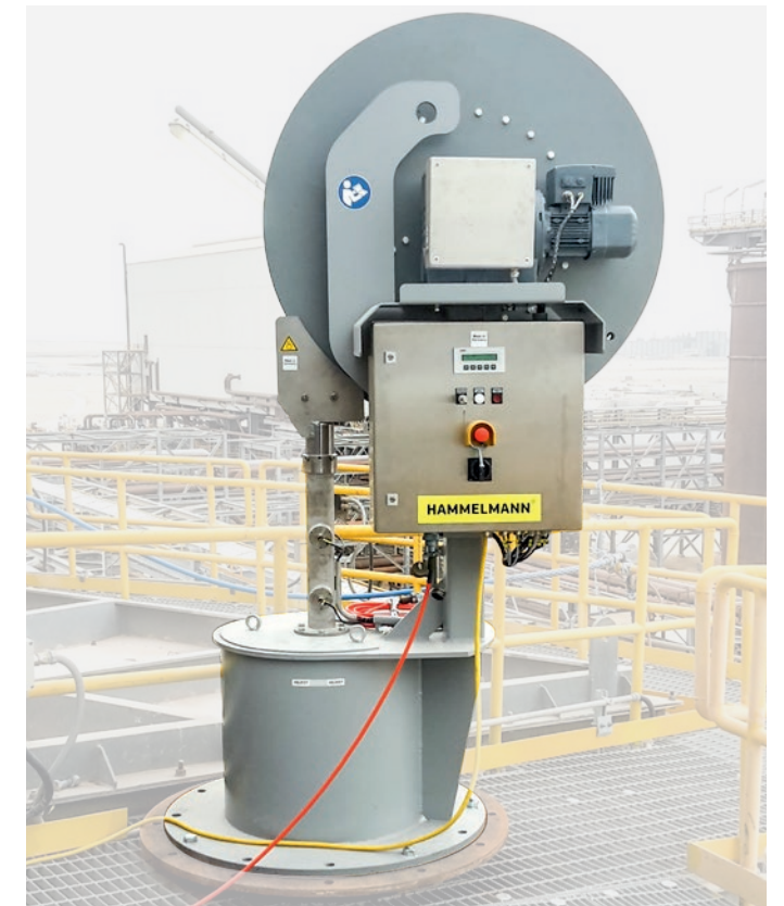
Hose reel system
