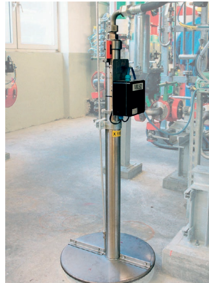
Lance system - moved hydraulically/pneumatically actuated
