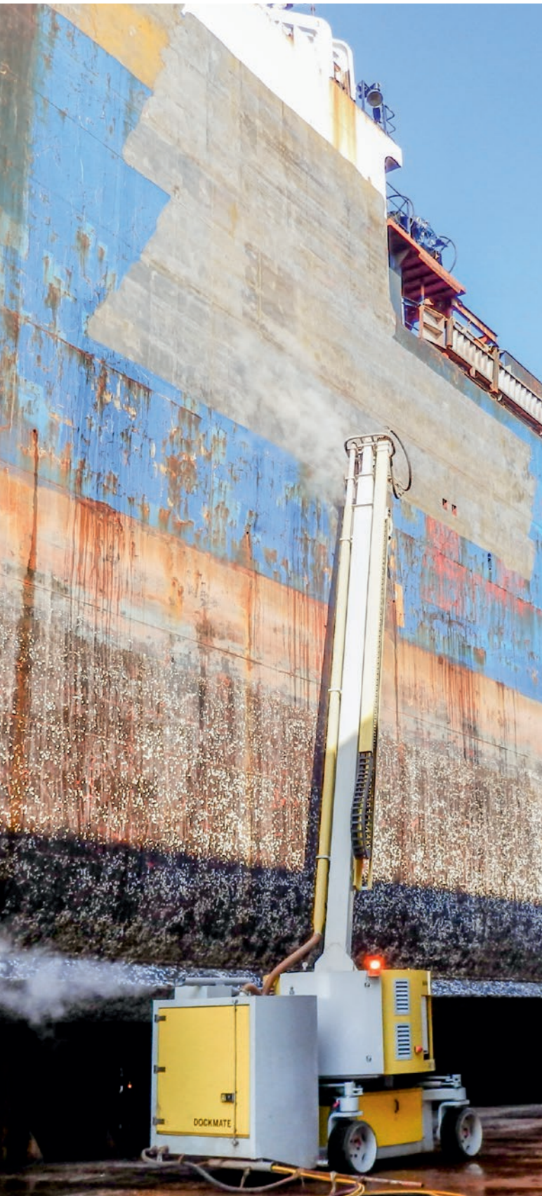
Dockmate - ship cleaning system
