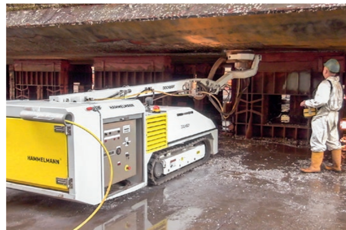
Dockboy - surface preparation on ship hull bottoms
