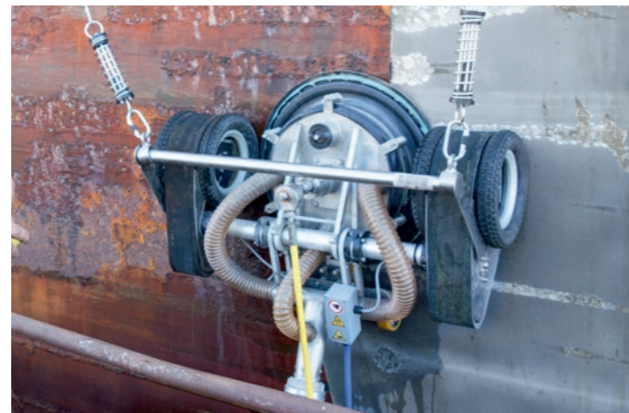
Spiderjet M - magnetically adhering surface cleaning device
