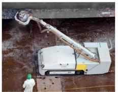
In combination with direct vacuuming, it ensures eco-friendly rust removal and old coating removal with waste and waste water collection.
