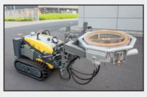
Self-sufficient carrier vehicle that can connect various jetting tools for surface treatment i.e. the cleaning and de-coating of ship decks,
