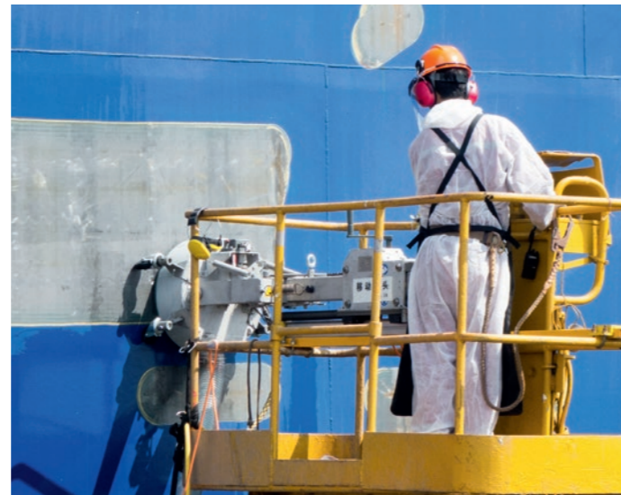
Aquablast Spot - to clean specific small areas
