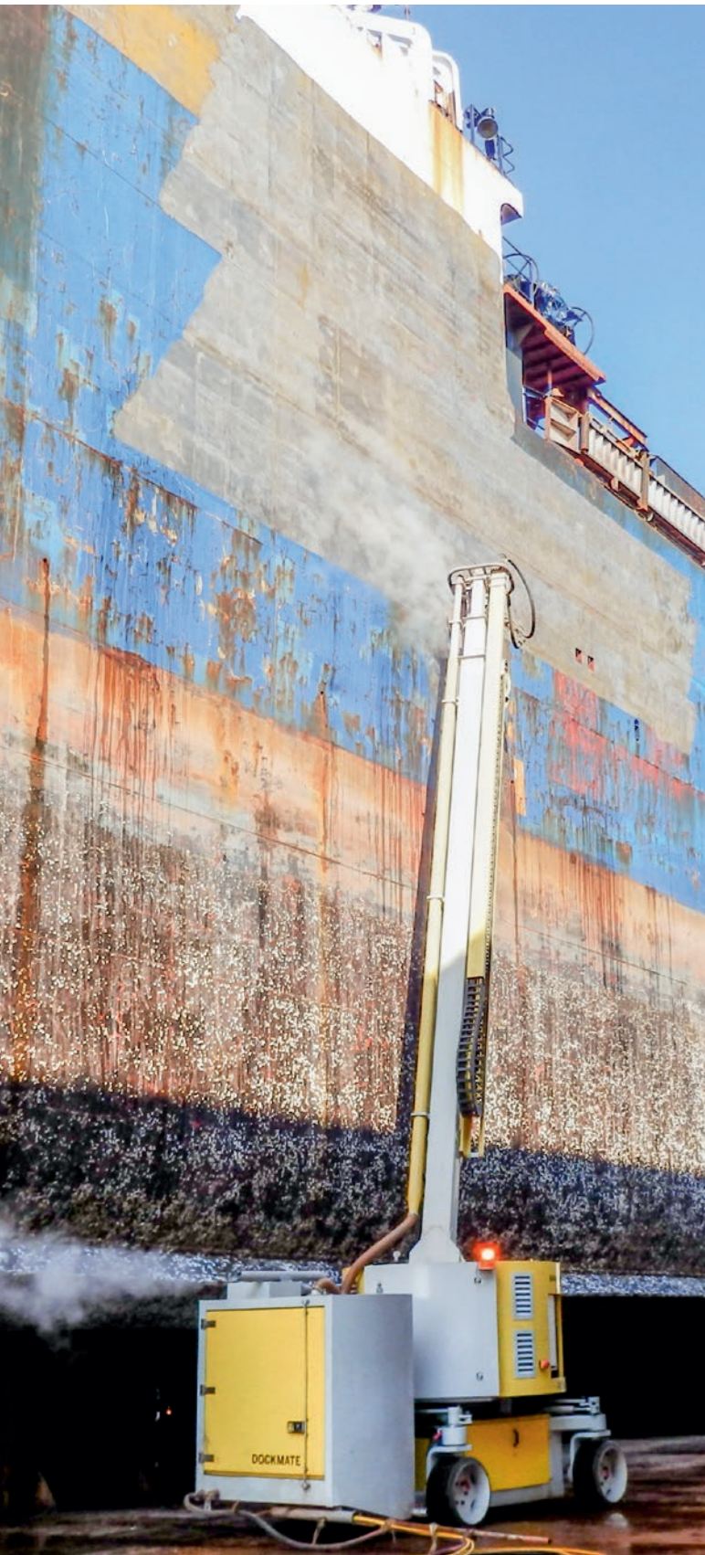
Dockmate - ship cleaning system
