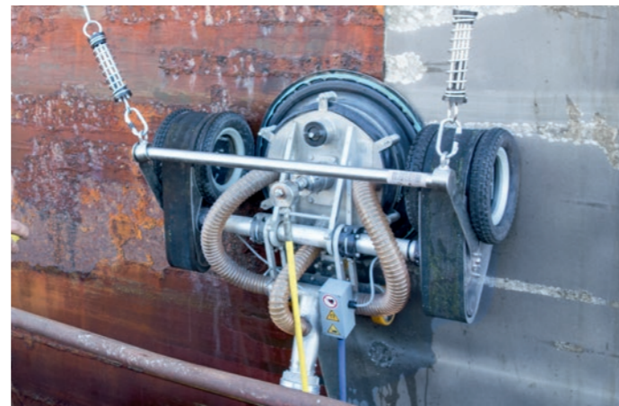
Spiderjet M - magnetically adhering surface cleaning device
