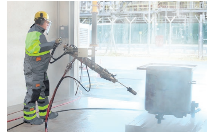
Jetmate - reaction force free jetting tool
