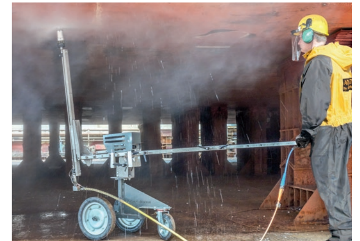
Jetboy - mechanical support for manual work
